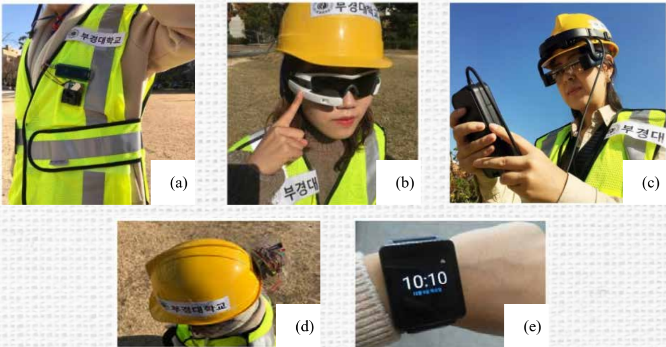
Figure 6. Proposed embedded wearable system shown at a mining site: (a) sensor-equipped mine safety vest; (b) miner wearing Recon Jet Smart Eyewear; (c) miner using Epson Moverio BT-2200; (d) sensor-equipped safety helmet; (e) smartwatch [28].
